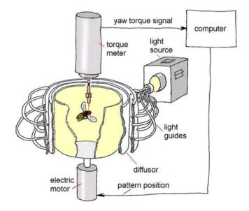
**Figure 2. Flight simulator set-up.** The fly is flying stationarily in a cylindrical arena homogeneously illuminated from behind. The fly's tendency to perform left or right turns (yaw torque) is measured continuously and fed into the computer. In closed-loop, the computer controls arena rotation (single stripe or uniform texture as patterns on the arena wall). An additional white screen (not shown) covered the arena from above for all groups. doi:10.1371/journal.pone.0000443.g002
